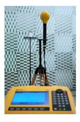
First, the frequency and transmission behaviour in the different operating states (see Paragraph 1.4 Definitions) of standby mode, standby mode incl. connectivity check and active mode is determined. The operating states are achieved here using suitable settings or applications (e.g. external noise source).
